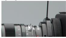
4) Use the widest lens you have available, as wider lenses are more sensitive to flange focal length. Open the aperture of the SLR lens all the way and set the focus ring on your 35mm lens to 3 feet.
