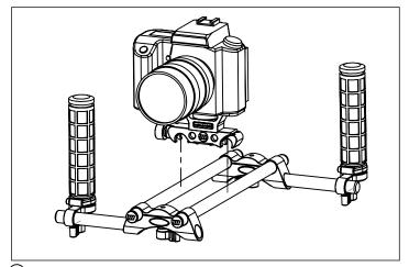
4 Attach Camera / DSLR Baseplate Assembly to CF Support Rods
