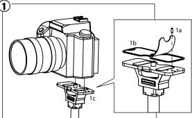
(1a) Attach camera specific set screw to DSLR Baseplate. Kit comes with Canon and Nikon set screws (1b) OPTIONAL LIP PAD Assembly
